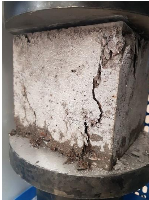
Figure 3. Failure of a concrete specimen
